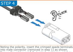
into male connector (removed in step 1) as shown. Ensure the cables are fully located - retaining catches will click into place.
