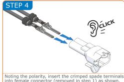
Noting the polarity, insert the crimped spade terminals into female connector (removed in step 1) as shown. Ensure the cables are fully located - retaining catches will click into place.
