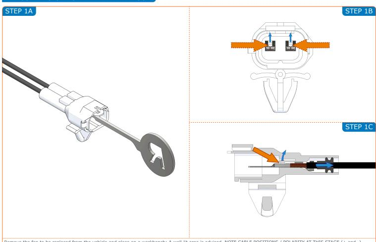
Remove the fan to be replaced from the vehicle and place on a workbench; A well-lit area is advised. NOTE CABLE POSITIONS / POLARITY AT THIS STAGE (+ and -). Insert the supplied pin removal tool between the male spade and the retaining lug. Use slight force to lever the retaining lugs as shown above. The cables may need to be pushed inwards to relieve pressure on the lugs to allow removal. Step 1A and 1B show the lugs from the front and as a section view through.
