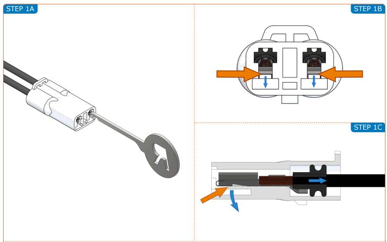
Remove the fan to be replaced from the vehicle and place on a workbench; A well-lit area is advised. NOTE CABLE POSITIONS / POLARITY AT THIS STAGE (+ and -). Insert the supplied pin removal tool between the female terminal and the retaining lug. Use slight force to lever the retaining lugs as shown above. The cables may need to be pushed inwards to relieve pressure on the lugs to allow removal. Step 1A and 1B show the lugs from the front and as a section view through.
